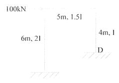
Q.4(A) Analyse the frame given below by matrix stiffness method. The area of each member given in parenthesis in mm<sup>2</sup>. Take E=200 KN/mm<sup>2</sup>. The height of the frame is given as 1m.
